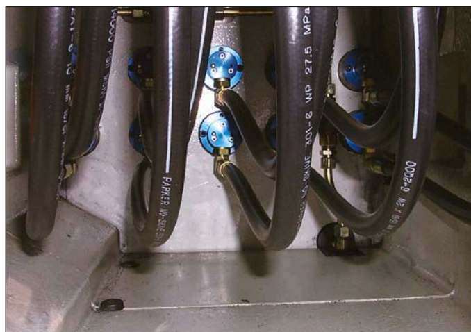
Deublin 1117 Bearingless Unions on Automotive Transfer Line.
